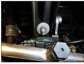
5. Remove the nut that secures intake plenum to the engine and then remove the intake plenum from the vehicle.
